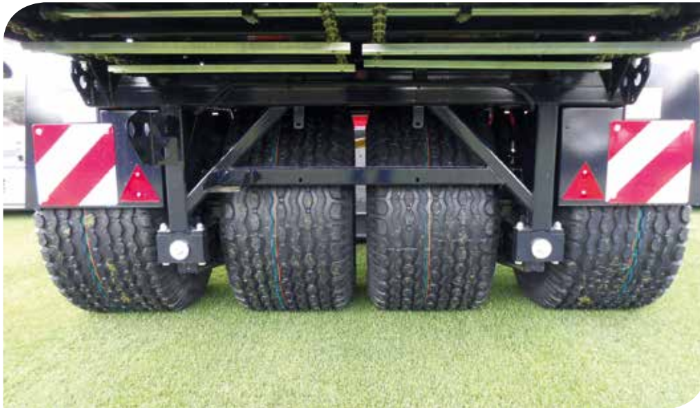
Prevent ruts and tire marks with extra wide tires and the optional Pendle axle.
