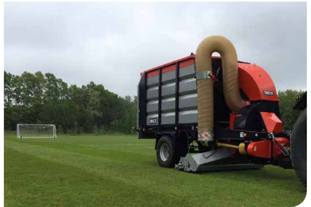
Every TRILO vacuum sweeper can be fitted with a suction hose with the exception of vacuum sweepers that are fitted with wings.
