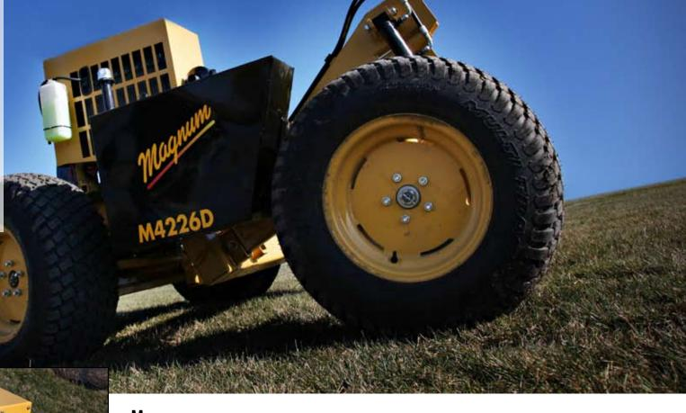
**M**eet Magnum's latest Installer, the turf and operator friendly, four-wheel drive machine that combines efficiency and dependability into a conveniently compact package weighing less than 2000 pounds. The concept of this Installer grew out of the need for a lighter weight, quick moving vehicle for the installation of big rolls of sod, one that could handle the terrain but not damage the turf.
