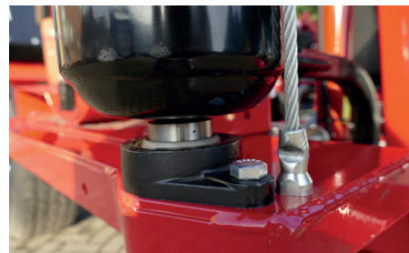
Maintenance free sealed bearings in both the blade spindles and roller ends.
