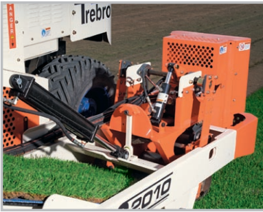
Floating head with adjustable-down-pressure
