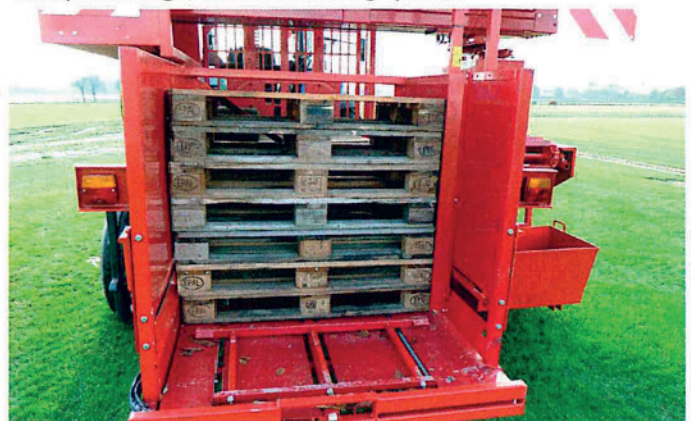
Palletinjector holds up to 7 pallets.
